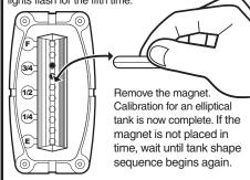
If the magnet is not placed in front of the display to select a tank shape, the tank selection sequence will continue and the FULL light will flash 5 times. After the FULL light flashes 5 times the tank shape selection sequence will begin again. (Step 5) The tank shape selection sequence will repeat 3 times. If no tank shape selection is made in this time, the display will default to a rectangular tank.
